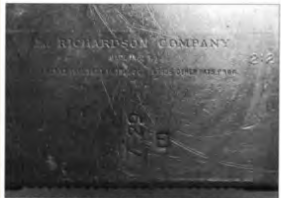
Figure 3. Bottom of a battery case showing the case supplier's logo and the battery manufacturer's identification letter and date of manufacture.
