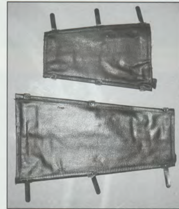
Spring covers. Each set consisted of two small covers for the front spring and two larger covers for the rear spring.
