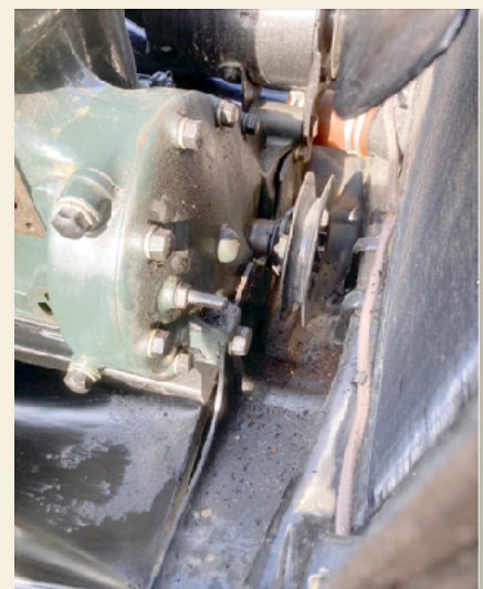
Fig. 163—Showing Where Engine Supporting Flange Plates of Ford Model A Old Style is Cut Away to Install New Flexible Support.
