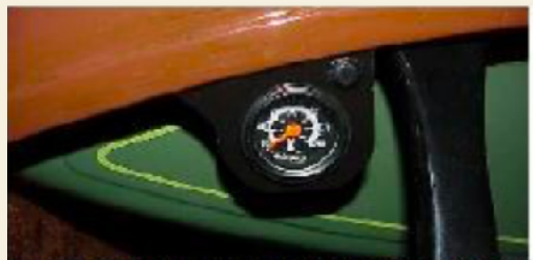
The little switch in the upper right corner of the bracket is a momentary push button switch wired to the meter that will give you a quick peek at the gauge while driving at night.
