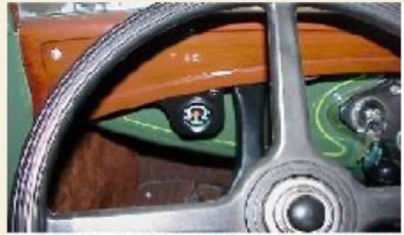
A 1 1/2" SunPro mechanical temperature gauge is installed with a custom made bracket up under the dash rail of a 1931 Victoria.
