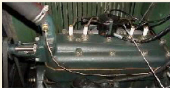
The six-foot mechanical cable is routed from the gauge to the Dan Eubanks reproduction water outlet casting that has been cast with a temperature gauge boss and has been drilled and tapped for your favorite size pipe fitting. 🚗
