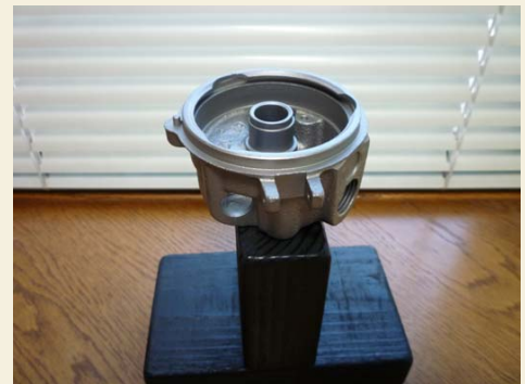
A cruddy swap meet distributor bead blasted and ready for masking and painting.
