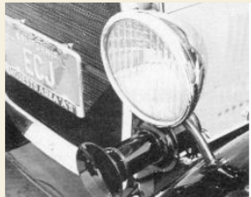
Chevy uses faceted reflectors and clear lens; Ford used smooth reflectors and gridded lenses.
