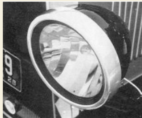
Chevy uses faceted reflectors and clear lens; Ford used smooth reflectors and gridded lenses.
