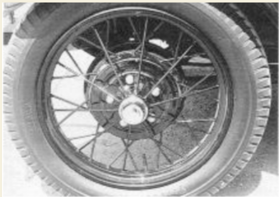
The A's welded steel spokes give cars a rich lighter appearance than the heavy Chevy disc,
