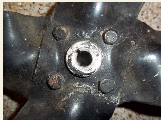
Four-bladed fan welded across blade roots.
