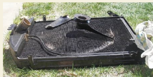
Damaged radiator showcasing copper smile. Photo: Steve Schullery
