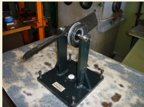
Fan balancing apparatus utilizing ball bearings. Photo: Tom Endy
