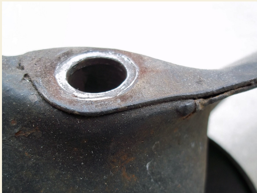
Non welded area susceptible to cracks. Start of a crack can be seen on the right side
