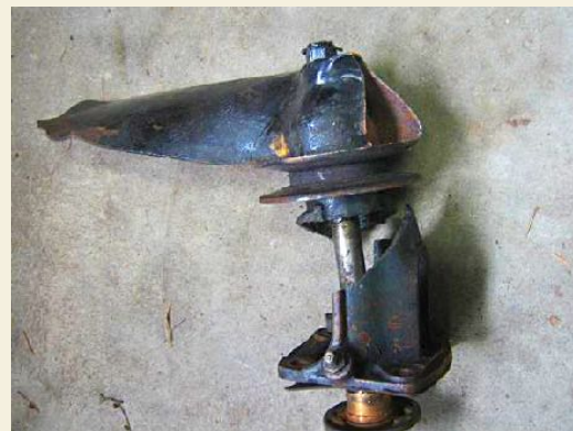
Broken water pump housing and fan. Photo: Don Bader
