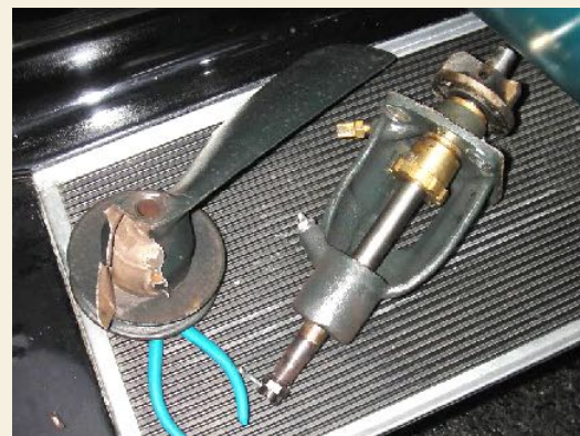
Broken fan; notice the hollow hub. Photo: Steve Schullery
