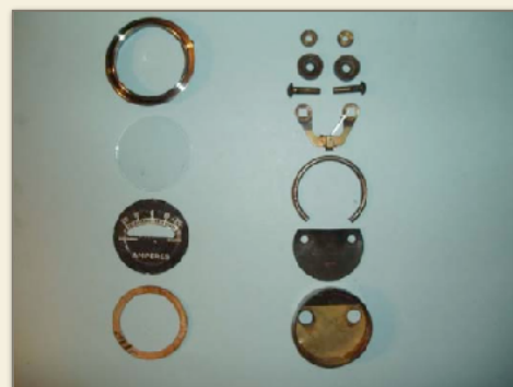
The Model A ammeter is a fairly simple device
