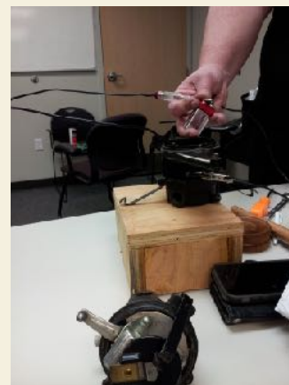
Setting the distributor the traditional way.
