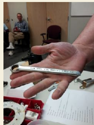
Special tool Clyde made for the distributor cam.
