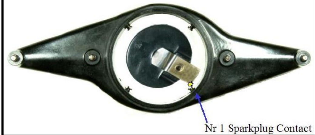
Rotor Position, Spark Lever Up, Timing at TDC
