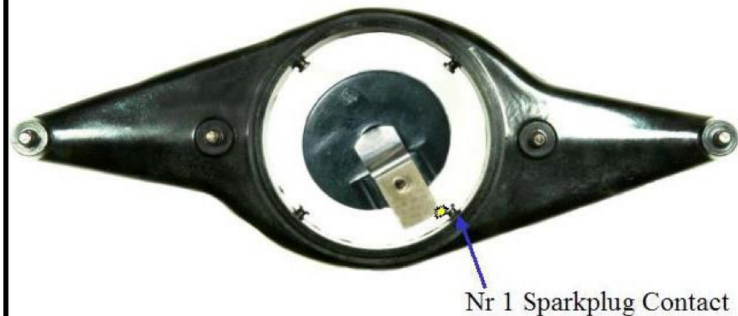
Rotor Position, Spark Lever Down, Timing at 40° BTDC
