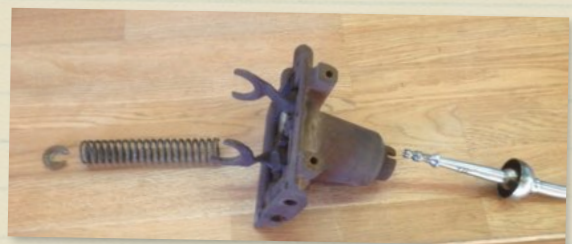
This is the order of the parts that make up the gear shift part of the tower - note the spring and keeper that clips onto the stick to hold it tight.
