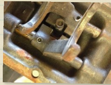
You can see how the shift stick ball interacts with the fork notches - the tighter the ball fits in the notches the less slop will exist in the shifter - there does need to be some play however so that you can still shift smoothly.
